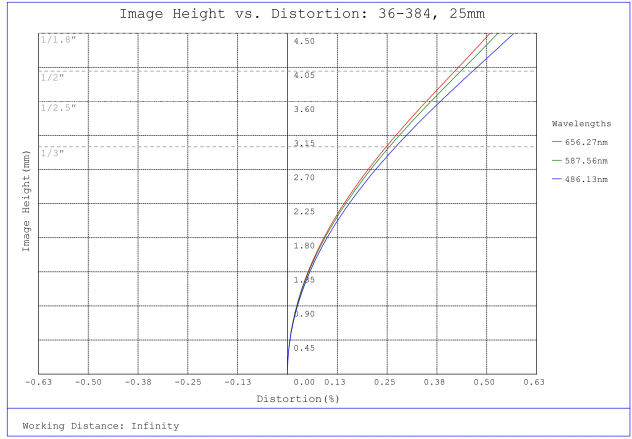
#36-384, 25mm FL f/2.5, Rugged Blue Series M12 Lens, Distortion Plot
