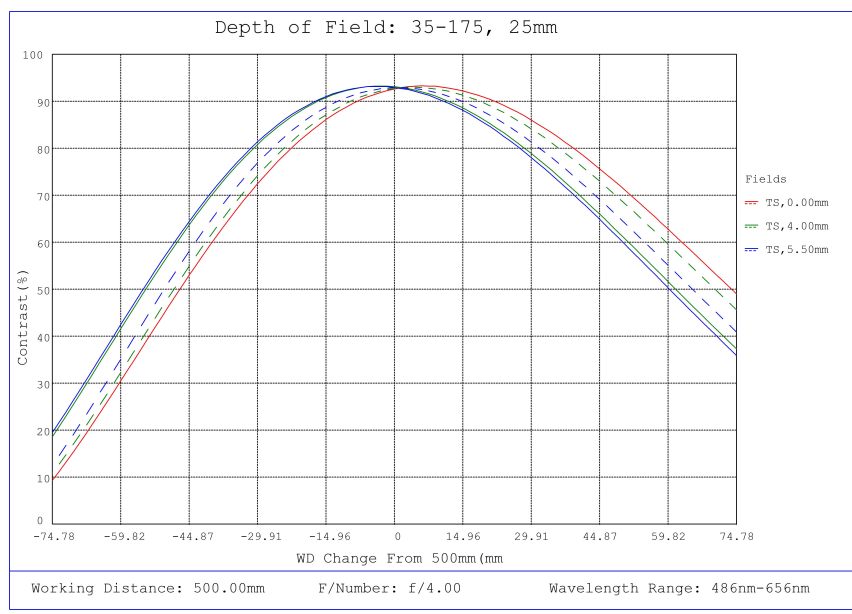
#35-175, 25mm, f/4 Cr Series Fixed Focal Length Lens, Depth of Field Plot, 500mm Working Distance, f4
