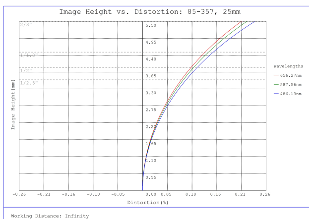
#85-357, 25mm, f/2.8 Ci Series Fixed Focal Length Lens, Distortion Plot
