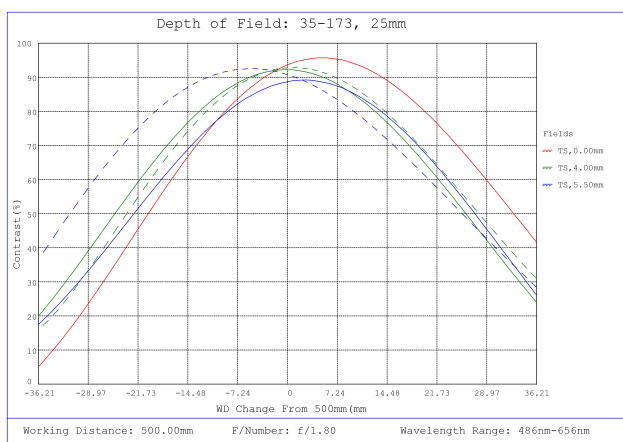
#35-173, 25mm, f/1.8 Cr Series Fixed Focal Length Lens, Depth of Field Plot, 500mm Working Distance, f1.8
