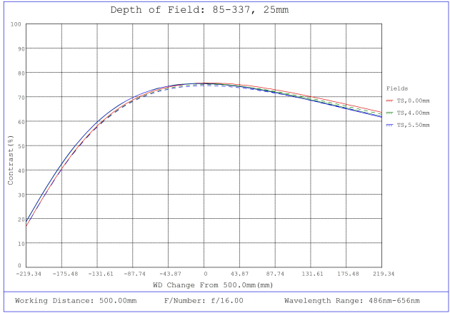
#85-337, 25mm, f/16 Ci Series Fixed Focal Length Lens, Depth of Field Plot, 500mm Working Distance, f16
