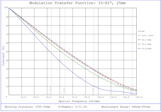
#33-827, 25mm f/11.0, HPi Series Fixed Focal Length Lens, Modulated Transfer Function (MTF) Plot, 1000mm Working Distance, f11
