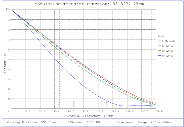
#33-827, 25mm f/11.0, HPi Series Fixed Focal Length Lens, Modulated Transfer Function (MTF) Plot, 500mm Working Distance, f11
