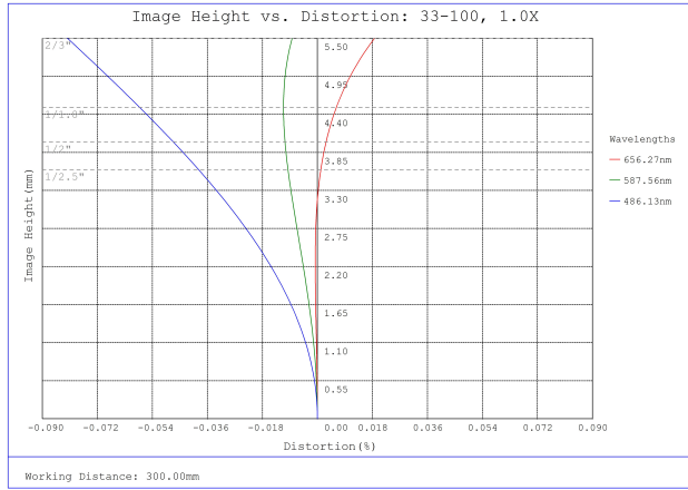
#33-100, 1X, 300mm WD CompactTL™ Telecentric Lens, Distortion Plot
