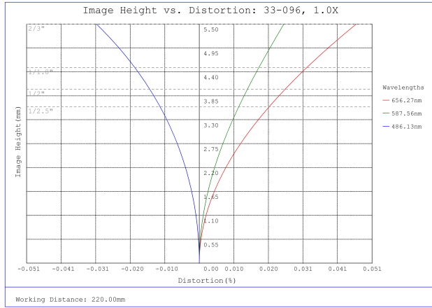
#33-096, 1X, 220mm WD CompactTL™ Telecentric Lens, Distortion Plot
