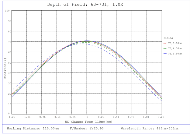
#63-731, 1X, 110mm WD CompactTL™ Telecentric Lens, Modulated Transfer Function (MTF) Plot, 110mm Working Distance, f20.9
