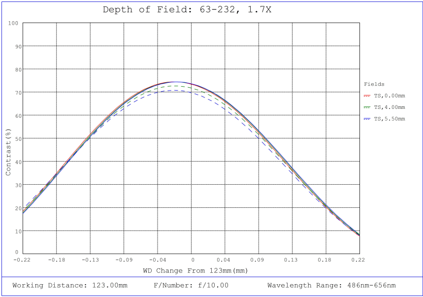
#63-232, 1.7X, 2/3" C-Mount PlatinumTL™ Telecentric Lens, Depth of Field Plot, 123mm Working Distance, f10
