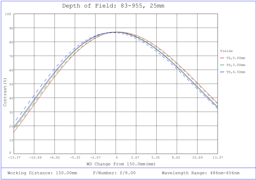
#83-955, 25mm FL f/8, Blue Series M12 Lens, Depth of Field Plot, 150mm Working Distance, f8
