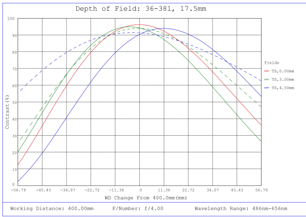
#36-381, 17.5mm FL f/4, Rugged Blue Series M12 Lens, Depth of Field Plot, 400mm Working Distance, f4
