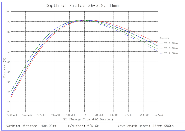
#36-378, 16mm FL f/5.6 Rugged Blue Series M12 Lens, Depth of Field Plot, 400mm Working Distance, f5.6
