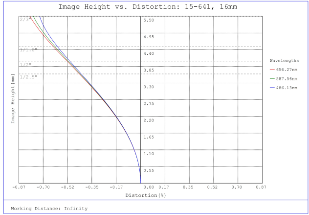
#15-641, 16mm, f/4 Cw Series Fixed Focal Length Lens, Distortion Plot
