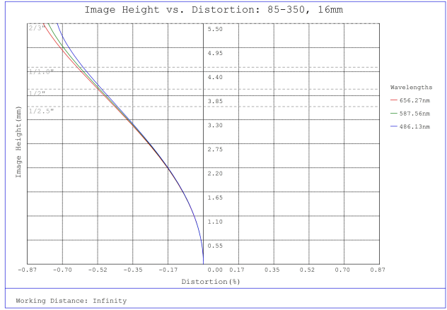
#85-350, 16mm, f/2.8 Ci Series Fixed Focal Length Lens, Distortion Plot
