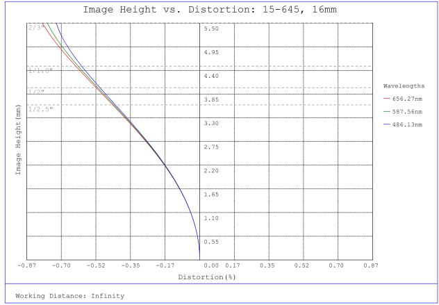
#15-645, 16mm, f/16 Cw Series Fixed Focal Length Lens, Distortion Plot
