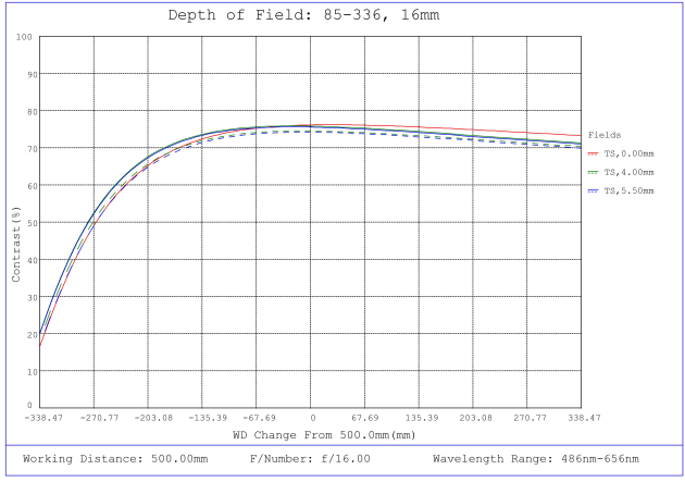
#85-336, 16mm, f/16 Ci Series Fixed Focal Length Lens, Depth of Field Plot, 500mm Working Distance, f16
