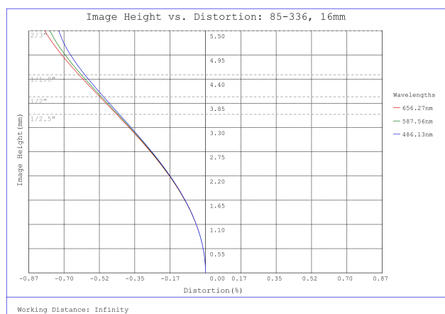
#85-336, 16mm, f/16 Ci Series Fixed Focal Length Lens, Distortion Plot
