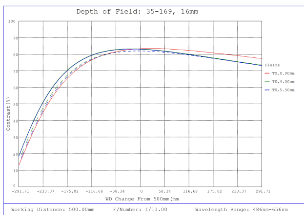
#35-169, 16mm, f/11 Cr Series Fixed Focal Length Lens, Depth of Field Plot, 500mm Working Distance, f11
