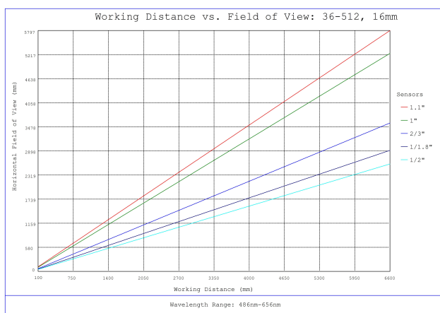
#36-512, 16mm f/2.8, HPr Series Fixed Focal Length Lens, Working Distance versus Field of View Plot
