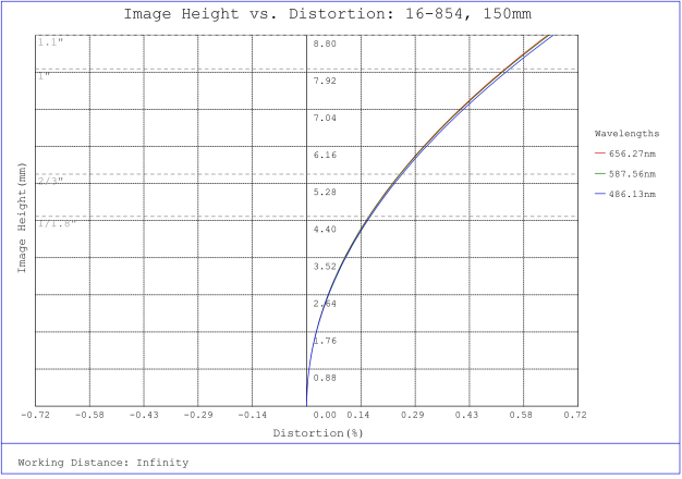
#16-854, 150mm, f/8 Athermal Lens, Distortion Plot
