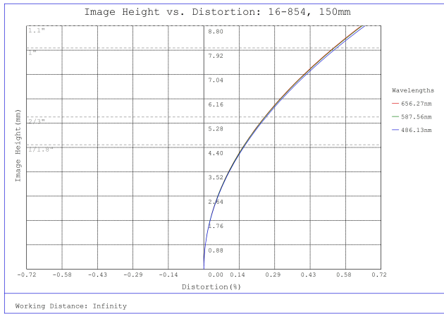
#16-854, 150mm, f/8 Athermal Lens, Distortion Plot
