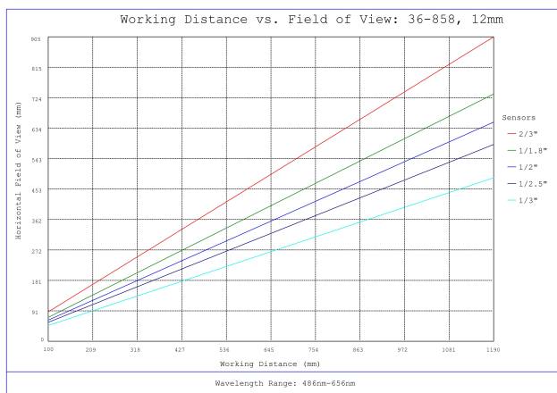
#36-858, 12mm f/8, 150-500mm Primary WD, HRr Series Fixed Focal Length Lens, Working Distance versus Field of View Plot
