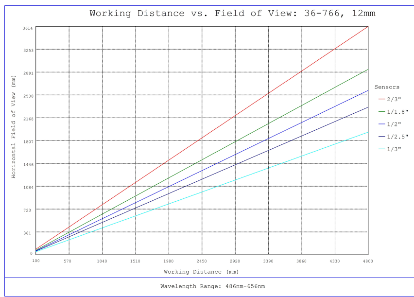
#36-766, 12mm f/8, 150-500mm Primary WD, HRi Series Fixed Focal Length Lens, Working Distance versus Field of View Plot
