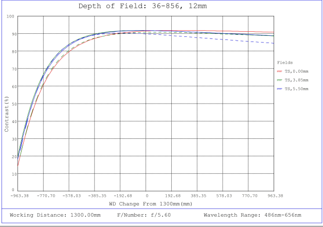
#36-856, 12mm f/5.6, 400-2000mm Primary WD, HRr Series Fixed Focal Length Lens, Depth of Field Plot, 1300mm Working Distance, f5.6
