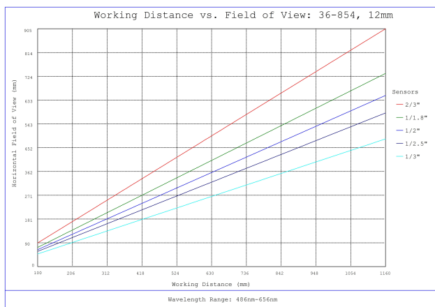
#36-854, 12mm f/4, 1000mm-∞ Primary WD, HRr Series Fixed Focal Length Lens, Working Distance versus Field of View Plot
