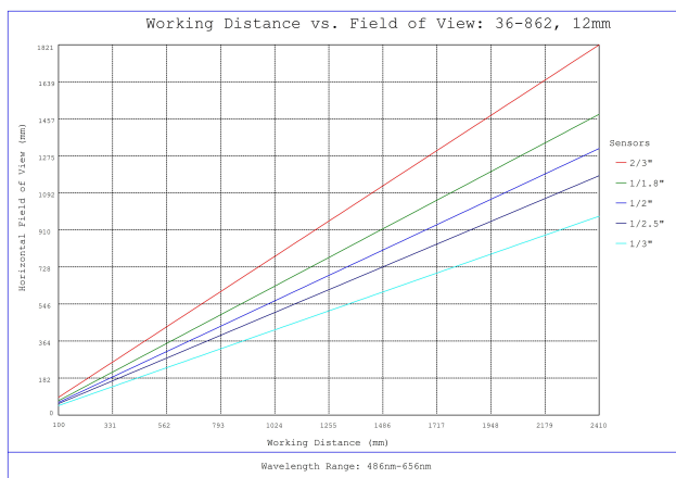
#36-862, 12mm f/11, 150-500mm Primary WD, HRr Series Fixed Focal Length Lens, Working Distance versus Field of View Plot
