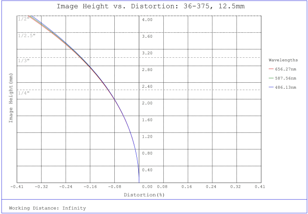
#36-375, 12.5mm FL f/8, Rugged Blue Series M12 Lens, Distortion Plot
