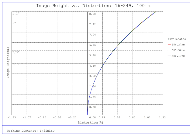
#16-849, 100mm, f/4 Athermal Lens, Distortion Plot
