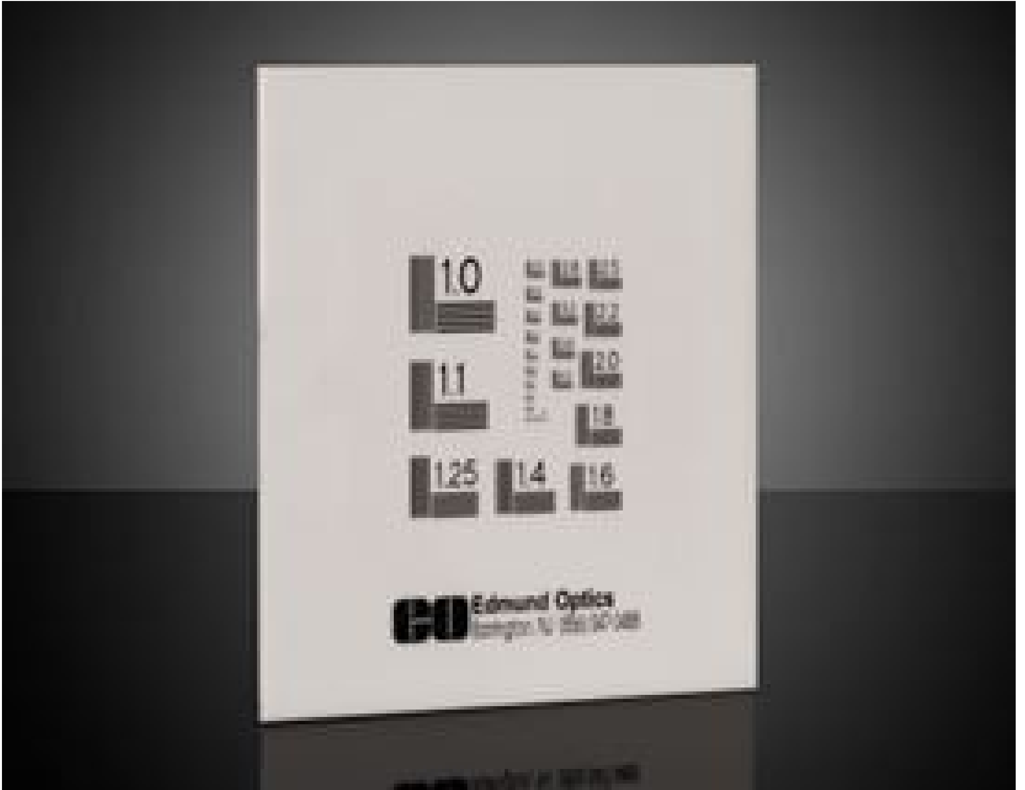
NBS 1963A Resolution Target
