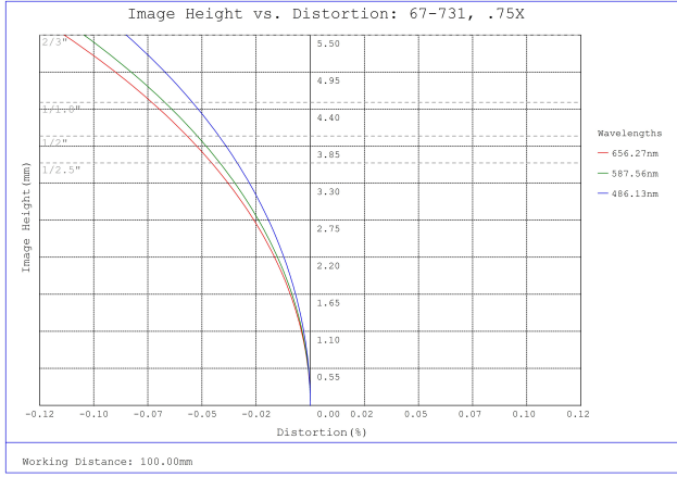
#67-731, 0.75X SilverTL™ Telecentric Lens, Distortion Plot
