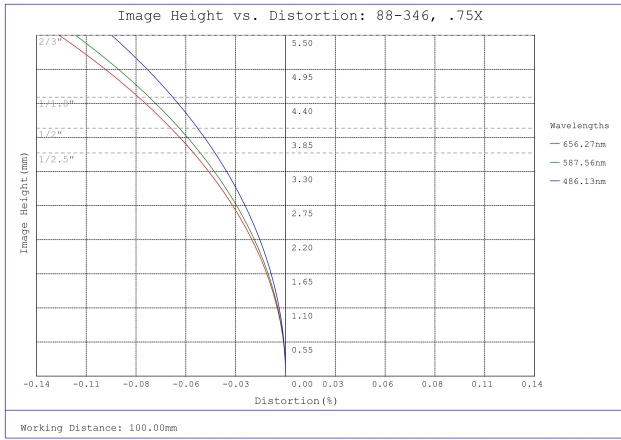
#88-346, 0.75X In-Line Illumination SilverTL™ Telecentric Lens, Distortion Plot
