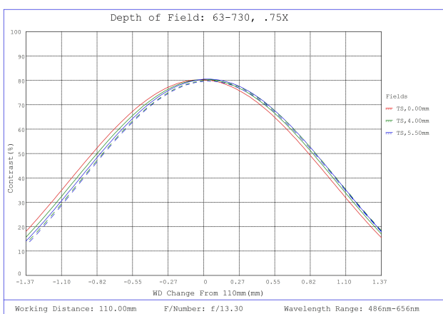
#63-730, 0.75X, 110mm WD CompactTL™ Telecentric Lens, Depth of Field Plot, 110mm Working Distance, f13.3
