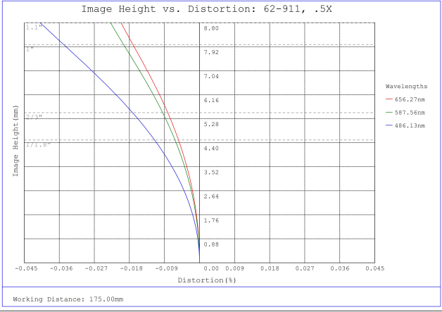
#62-911, 0.5X CobaltTL Telecentric Lens, Distortion Plot
