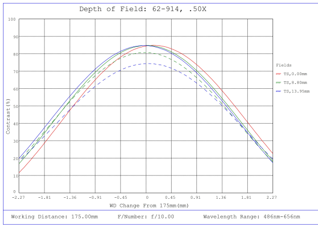
#62-914, 0.5X, 28.7mm M42 x 1.0 (19.53mm) PlatinumTL™ Telecentric Lens, Depth of Field Plot, 175mm Working Distance, f10
