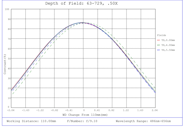
#63-729, 0.5X, 110mm WD CompactTL™ Telecentric Lens, Depth of Field Plot, 110mm Working Distance, f9.1
