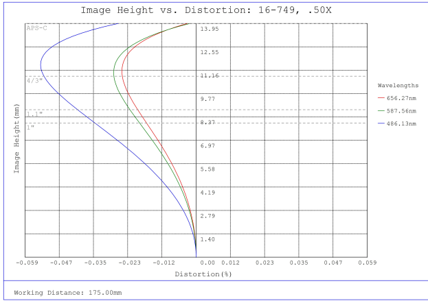
#16-749, 0.5X, 28.7mm TFL-Mount PlatinumTL™ Telecentric Lens, Distortion Plot
