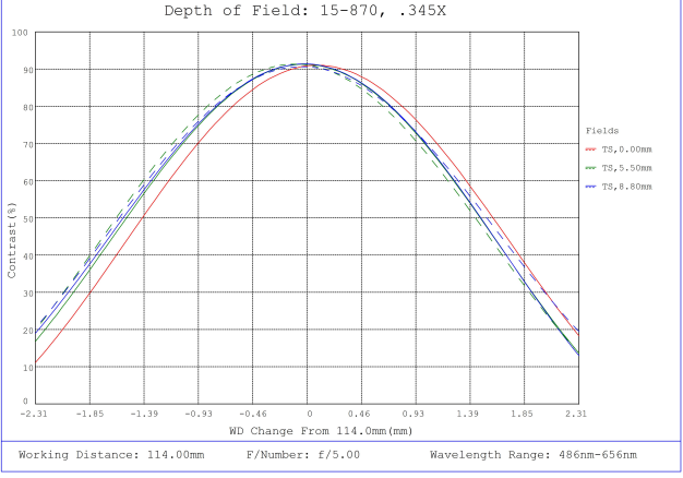
#15-870, 0.345X CobaltTL Telecentric Lens, Depth of Field Plot, 114mm Working Distance, f5
