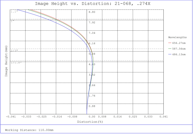
#21-068, 0.274X CobaltTL Telecentric Lens, Distortion Plot
