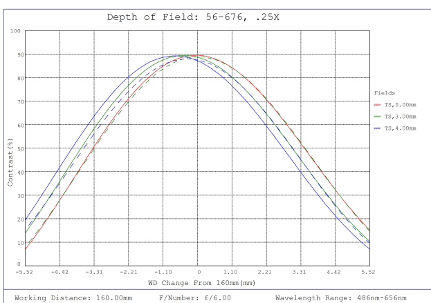
#56-676, 0.25X SilverTL™ Telecentric Lens, Depth of Field Plot, 160mm Working Distance, f6
