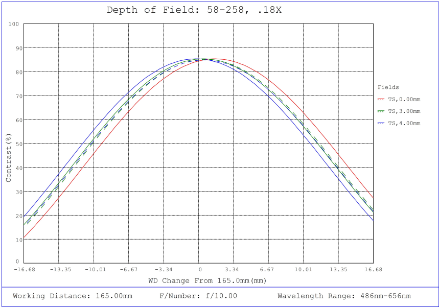
#58-258, 0.18X ½" GoldTL™ Telecentric Lens, Depth of Field Plot, 165mm Working Distance, f10
