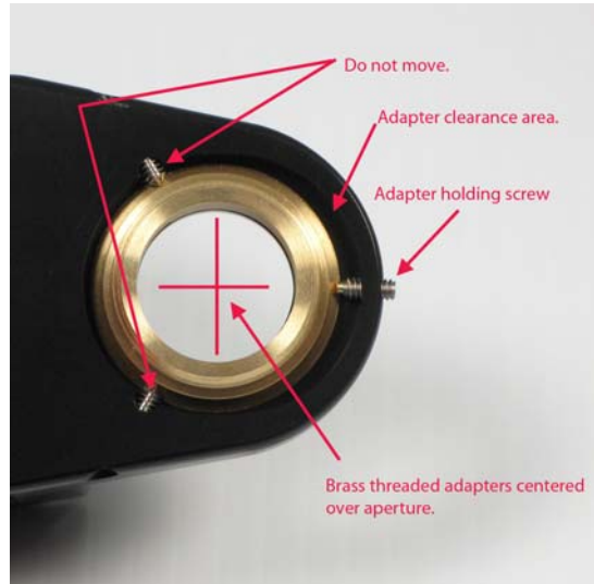
Figure 1: Bottom view of stage showing the male brass insert. Do not adjust the side set screws. Only the front set screw is adjustable.
