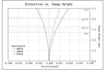
Figure 1: Distortion at the maximum sensor format. Positive values correspond to pincushion distortion, negative values correspond to barrel distortion.
