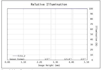
Figure 2: Relative illumination (center to corner)
