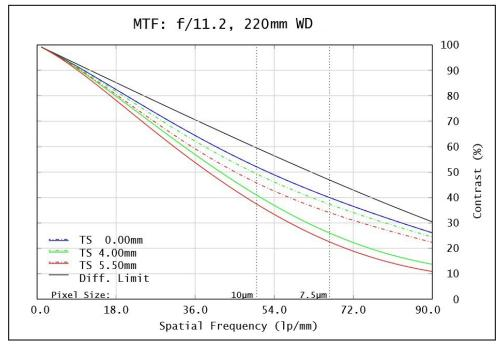
Figure 3: Image space polychromatic diffraction FFT Modulation Transfer Function (MTF) for λ = 486nm to 656nm. Included are the Tangential and Sagittal values for field points on center, at 70% of full field and the maximum sensor format. Solid black line indicates diffraction limit determined by f/#-defined aperture. Frequencies corresponding to the Nyquist resolution limit of pixel sizes are indicated.
