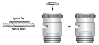
\*Appearance of Aperture for each focal length and f/stop may vary slightly, but the side of the aperture with the larger diameter hole is always the top.
