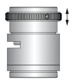
**5.** Thread entire assembly into C-Mount camera from the top of Rear Assembly until the top of the Locknut is flush against the camera C-Mount.
