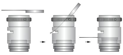
3. Using a spanner wrench, thread the bottom of Rear Assembly into the top of Main Housing until it is flat against the accessory, hand tightening torque or about 2.5-5kgf\*cm. If using a Liquid Lens, hold the Liquid Lens in place while tightening the Rear Assembly into Main Housing by inserting a paper-clip into one of the holes to the side of the Liquid Lens Holder. (Optional: spanner wrench #35-029 can be used)
