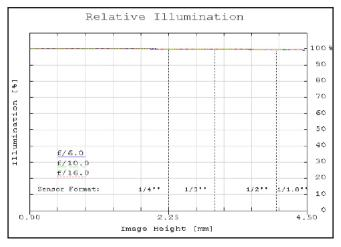
Figure 2: Relative illumination (center to corner)
