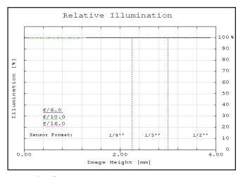
Figure 2: Relative illumination (center to corner)
