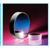
Substrate: Fused Silica **Dimensional Tolerance:** +0.00/-0.20mm Thickness Tolerance: ±0.20mm **Surface Accuracy:** 1/10λ Surface Quality: 20-10 Ground, 0.5mm max bevel Edges: Clear Aperture: Parallelism: 30 arcsec Commercial polish **Back Surface:**  $R_{avg} > 98\% @ 0 - 45^{\circ}$ , all polarizations Coating: >99% @ 0°, all polarizations
