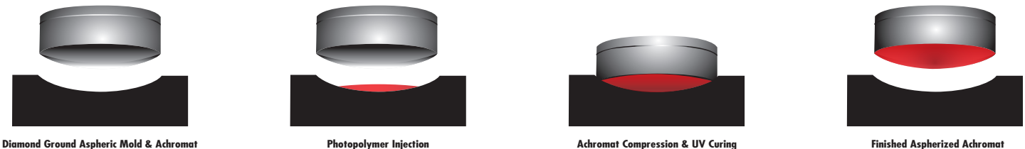
Figure 7: Aspherized Achromatic Lens Manufacturing
